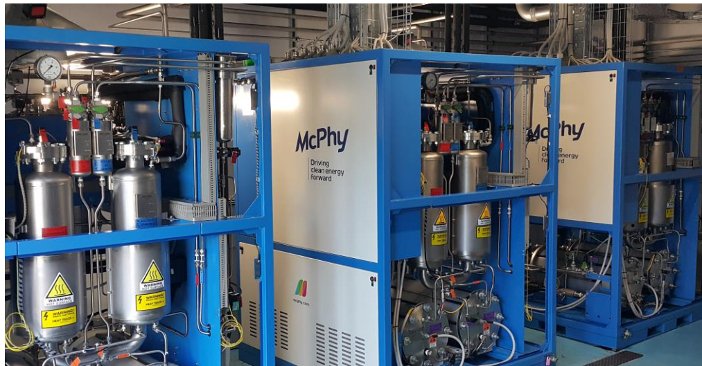
Industrial production unit of renewable hydrogen | Three McPhy's electrolyzers supplying 30 Nm 3 /h in nominal and 50 Nm 3 /h at peak.
