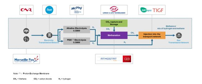
Ramping up of McPhy: deployment of innovative solutions at the heart of the global development of clean hydrogen as a key element of the transition to carbon-free energy
